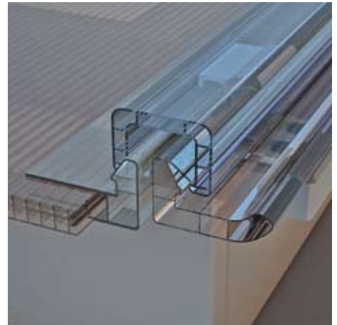
Detail of insertion of section-breaker profile to complete roofing.
