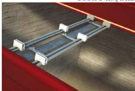
OVERLAP - STEP 1 Detail of double anchor bracket anchored to roofing structure
